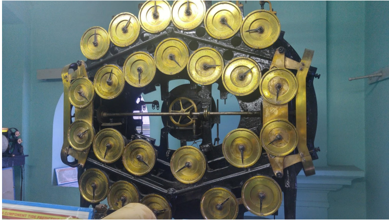
Left - 24 component tide predicting machine in use by the SOI from 1877 to 1952.
